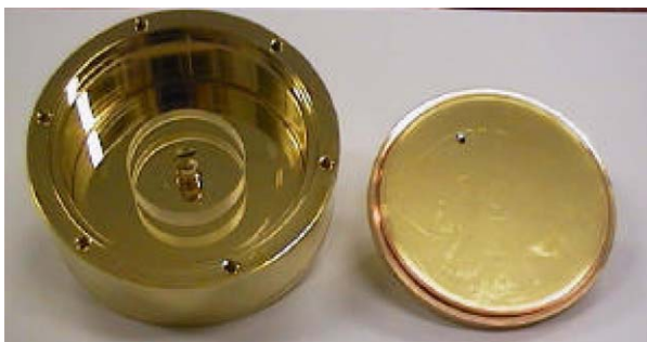
Fig. 2a : 26GHz-cavity before packaging
